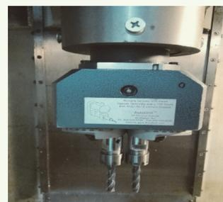
Twin spindle milling cutter adapter
