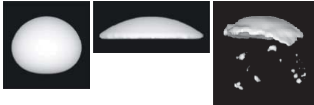
Fig. 1 Bubble motion rising in viscous liquids.
