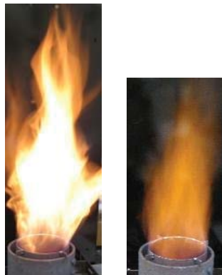
Fuel 100% Water 50vol% Fig.2 Burner flame
