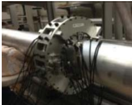
FIG. 2 Piezoelectric guided wave sensor system for piping inspection
