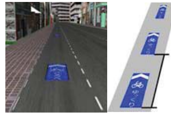
Repeated coloured sign syste,
