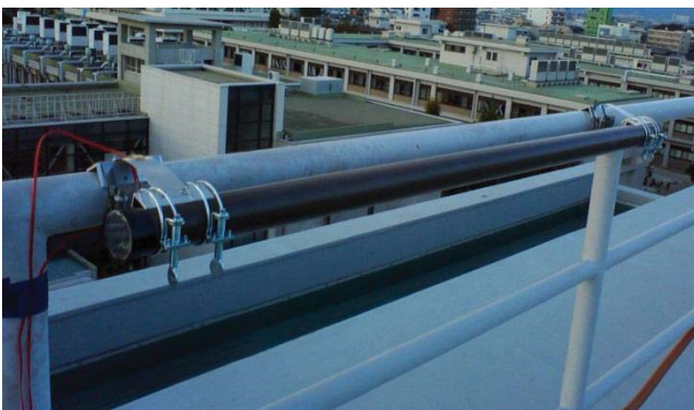
Fig. 2 Experiment of wake excitation behind railing of building roof for possibility of wind-generated electricity
